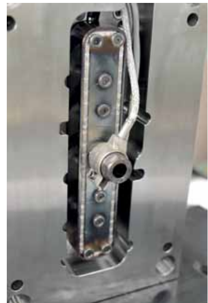
3/ 3D-printed manifold block for optimum flow paths
