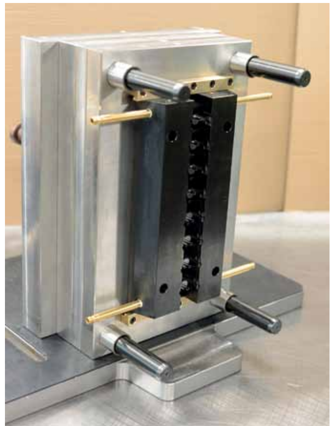
5/ Ejector half with DLC-coated slides
