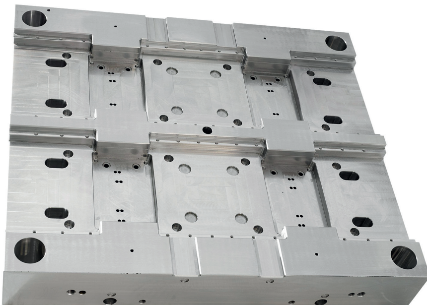
3/ Machining exclusively outside the cavity
