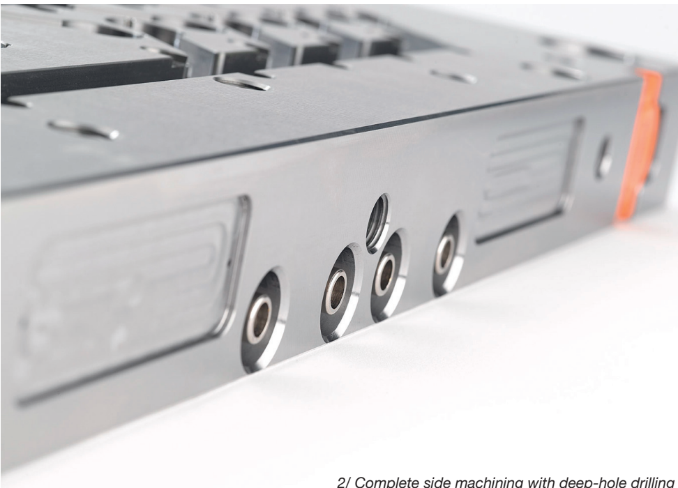
2/ Complete side machining with deep-hole drilling
