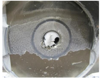
Figure 110: Incorrect height adjusting – insufficient preload
