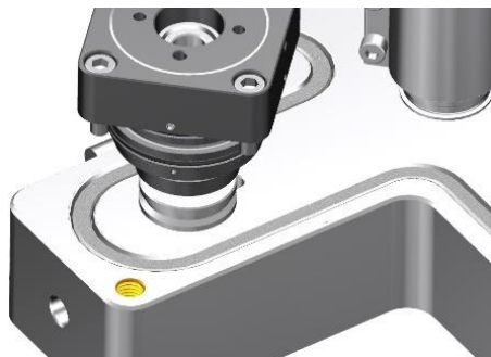
Figure 32: Transport thread on a hot runner
