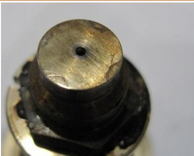
Figure 111: Leakage due to contact of the nozzle melt chamber
