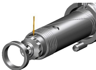
Figure 60: External TC Vario Shot shaft heater
