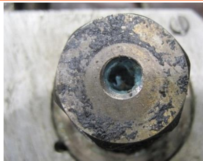
Figure 112: Nozzle contact radius not aligned, leakage possible
