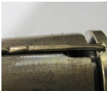
Figure 95: Defective / squeezed thermocouple element
