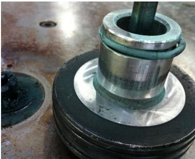
Figure 108: Piston seal defective
