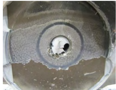
Figure 110: Incorrect height adjusting – insufficient preload
