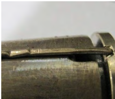
Figure 95: Defective / squeezed thermocouple element
