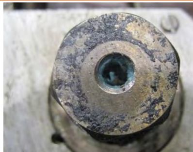
Figure 112: Nozzle contact radius not aligned, leakage possible
