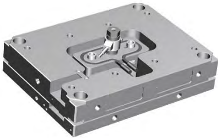
Figure 40: Mounted hot runner
