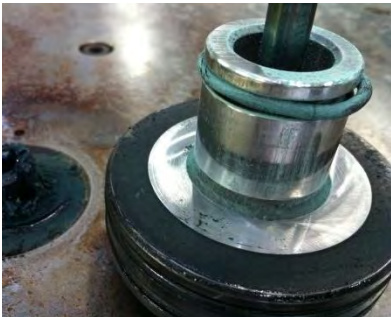
Figure 108: Piston seal defective
