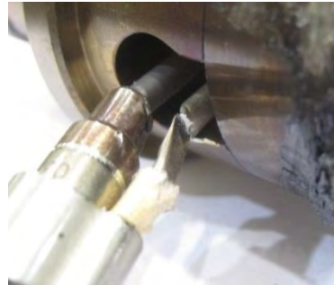
Figure 93: Defective / severed thermocouple element
