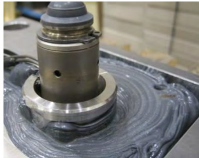
Figure 109: Incorrect height adjusting – hot runner covered in plastic
