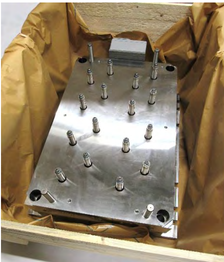
Figure 31: Hot half on the pallet after the protective caps have been removed
