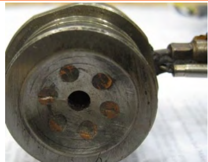
Figure 113: Damaged sealing surface on the contact radius, leakage possible
