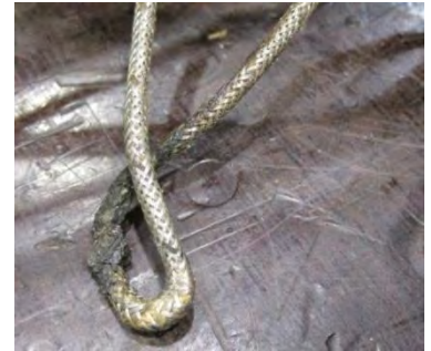
Figure 94: Squeezed heater cable
