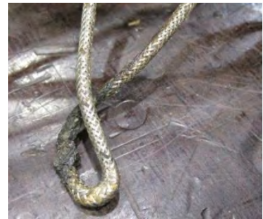
Figure 76: Squeezed heater cable
