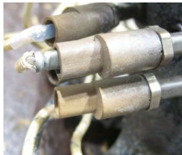
Figure 78: Torn-off heater cables, too small a bending radius
