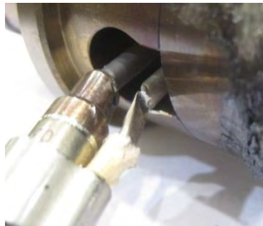
Figure 75: Defective / severed thermocouple element
