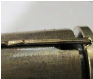
Figure 77: Defective / squeezed thermocouple element
