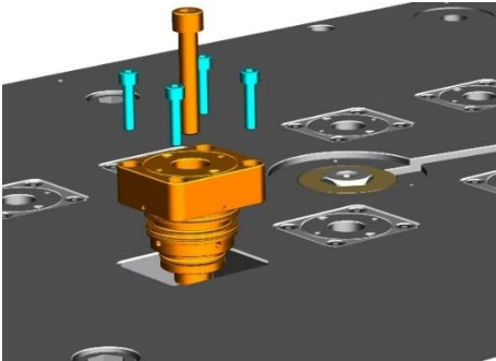
Figure 59: Mounting the actuation unit
