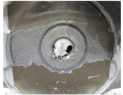
Figure 110: Incorrect height adjusting – insufficient preload
