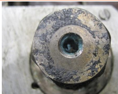
Figure 112: Nozzle contact radius not aligned, leakage possible
