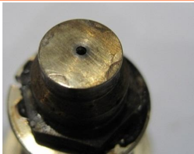
Figure 111: Leakage due to contact of the nozzle melt chamber
