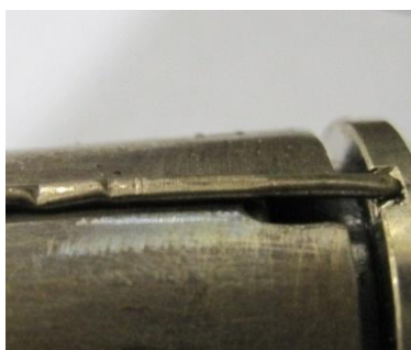
Figure 95: Defective / squeezed thermocouple element
