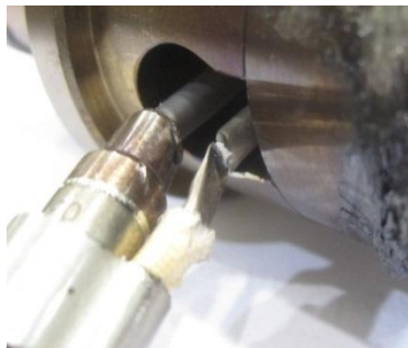
Figure 93: Defective / severed thermocouple element
