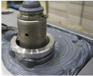
Figure 109: Incorrect height adjusting – hot runner covered in plastic
