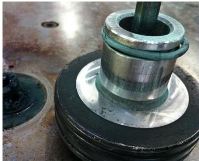
Figure 108: Piston seal defective
