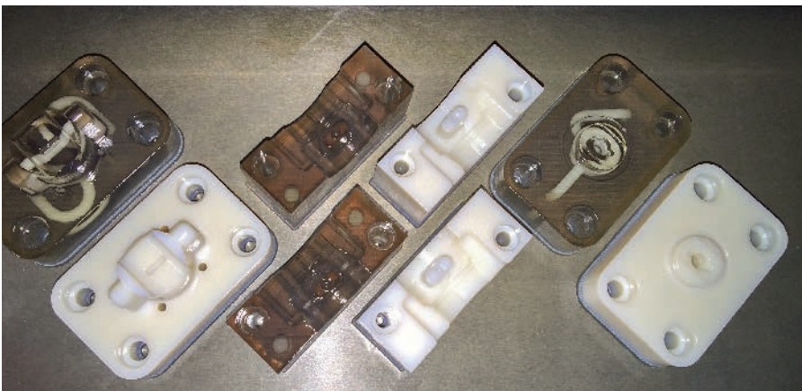
Cavity parts in „Digital ABS“ 3D printed by the Polyjet process!
