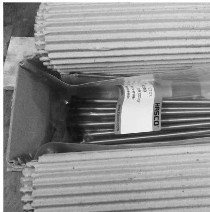
Individual parts packed in cardboard, plastic bag and corrugated board for protection
