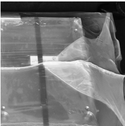
Sheets on pallet with cardboard underlay, fastener straps and shrink film
